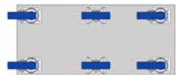
Four swivel castors and two fixed castors identical mounting height
