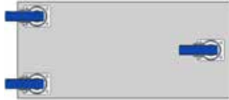
Three swivel castors with identical mounting height
