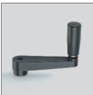
Square hole. Rotating cylindrical handle. Za: Zinc die-cast, plastic coated, black. AL: Aluminium, plastic coated, black. Cylindrical handle: Black Phenolic. Alternative to crank handles DIN 469.
